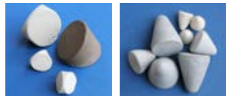
Examples of non-chipping ceramic media shapes are cylindrical wedges (left) and cones (right), neither of which have sharp, protruding edges.
