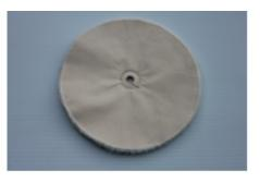
**Concentric Sewn** buffs also referred to as a Jewelers buffs are a buff that are sewn in round 1/2" to 1" increments. These buffs are firmer than a loose finishing buff, and sometimes are used as a minor cut buff. The buff sewn seems are commonly cut when reached to expose the next softer amount of material. The concentric sewn buff is produced in 1/2" to 1" widths which is also determined by the number of plies. This
