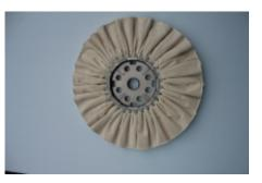
yellow maze. Each buff manufacturer will have 3-4 standard to specialized colored dip treatments that will also vary in hardness. The Airway buff is the standard buff for production buffing whether it be a manual or automated process. The buff can cut or finish all metals and composites.
