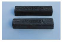
**Tripoli** is a cut compound used in softer metals, plastics and composites. The abrasive is a tripoli (micro crystaline structure) classified as a silica from a mine that is crushed and finely graded. Tripoli is a good cutting compound for aluminum, brass, copper, zinc, plastics and soft composites.
