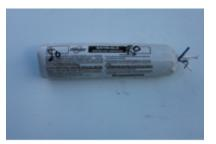
**Stainless compound** are a cut compound used for harder metals. It has a tallow(animal fat) binder with 150 to 400 grit aluminum oxide abrasive (blocky structure). The binder can be produced to be dry or greasy. The greaser the compound the faster the cut. There is a light grey(Dryer) version and a darker grey(greaser) version. Stainless compound is an excellent choice for steel and stainless steel cut buff applications.
